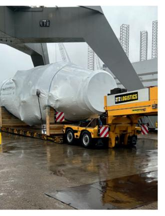
An excellent example of a complex task is transporting four pile clusters (measuring 15 x 12.25 x 12 metres and weighing 207 tonnes each) from the production site to shipment at the Port of Aabenraa.
