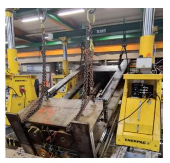
four Enerpac SL400Ns are narrow-bodied gantries for heavy lifts in tight spaces. These hydraulic towers provide a maximum capacity of 400 tonnes. However, the
