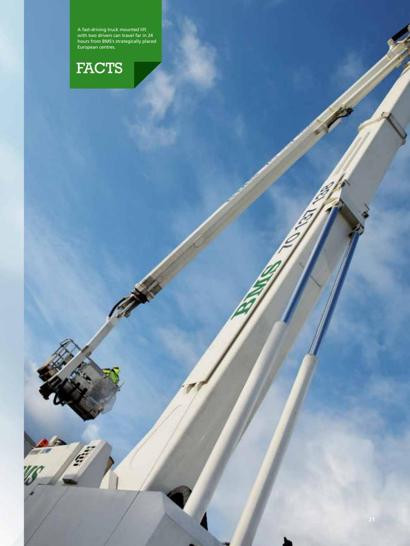
All BMS-cranes are equipped with two winches in order to turn elements in the air, regardless if they weigh one or 40 tonnes
